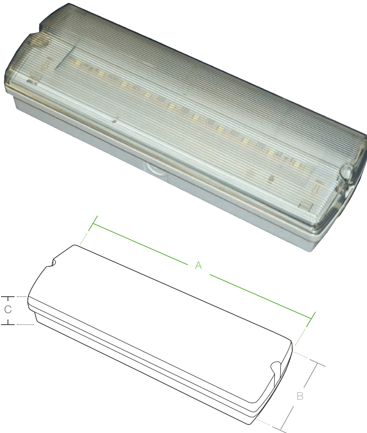
ERLED Dimensions: A: 346mm B: 105mm C: 78mm
